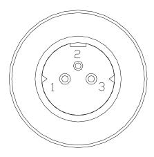
Pin 1: Vcc Pin 2: GND Pin 3: PWM
