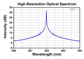
This high-resolution optical spectrum is obtained using one of Thorlabs' Optical Spectrum Analyzers (OSA201), which provides 8 pm resolution at 852 nm.
