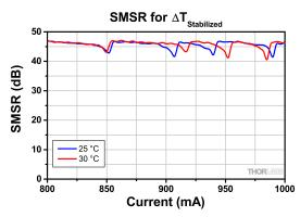
The typical side mode suppression ratio (SMSR) is shown for three temperatures within the wavelength stabilized temperature range  $(\Delta T_{\text{Stabilized}})^*$ .
