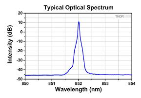
The typical optical spectrum is shown above. The data was obtained with a 1000 mA drive current and the device held at 25  $^{\circ}$ C.
