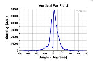
The diverging beam from the laser chip freely propagates through the external volume holographic grating (VHG), while the light in the center of the beam is reflected back into the chip. This results in a stabilized wavelength emitting from the laser and also creates a dark spot in the far field, as shown in the graphs above.
