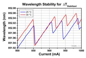
When used within the wavelength stabilized temperature range ( $\Delta T_{Stabilized}$ )\*, the LD852-SEV600 shows excellent wavelength stability over a range of drive currents.
