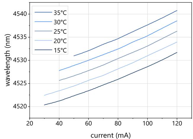
Typical mode hop free tuning of a nanoplus DFB ICL at 4524 nm by current and temperature
