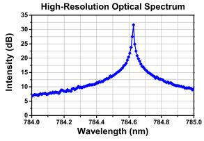
This high-resolution optical spectrum was obtained using one of Thorlabs' Optical Spectrum Analyzers (OSA201), which provides 8 pm resolution at 785 nm.
