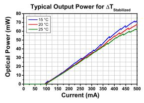
The typical output power vs. current is shown for three temperatures within the wavelength stabilized temperature range  $(\Delta T_{Stabilized})^*$  of a LP785-SAV50 laser diode.
