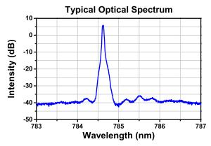
The typical optical spectrum is shown above. The data was obtained with a 400 mA drive current and the device held at 25 °C.
