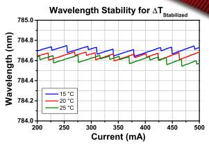
When used within the wavelength stabilized temperature range  $(\Delta T_{Stabilized})^*$ , the LP785-SAV50 shows excellent wavelength stability over a range of drive currents.
