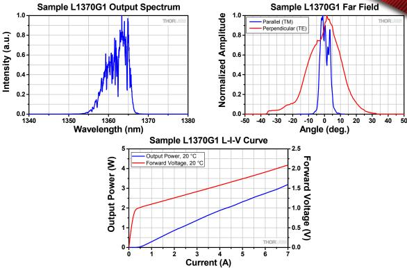
The data presented here is for one particular laser diode. Slight variations in performance data will occur from device to device. The sample spectrum and L-I-V spectrum of the L1370G1 laser diode was taken at 20°C. The far field was measured at a distance of 7" from the diode.
