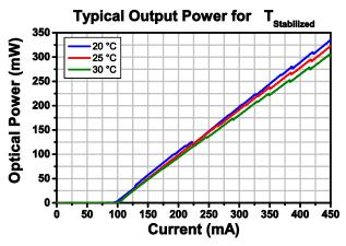
The typical output power vs. current is shown for four temperatures within the wavelength stabilized temperature range  $(\Delta T_{Stabilized})^*$  of a LD785-SEV300 laser diode.
