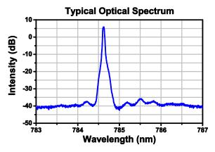
The typical optical spectrum is shown above. The data was obtained with a 500 mA drive current and the device held at 25 °C.
