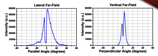
The diverging beam from the laser chip freely propagates through the external volume holographic grating (VHG), while the light in the center of the beam is reflected back into the chip. This results in a stabilized wavelength emitting from the laser and also creates a dark spot in the far field, as shown in the graphs above. These were measured with a current of 500 mA.
