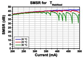
The typical side mode suppression ratio (SMSR) is shown for three temperatures within the wavelength stabilized temperature range  $(\Delta T_{\text{Stabilized}})^*$ .
