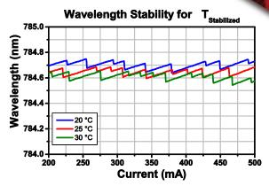
When used within the wavelength stabilized temperature range (ΔT<sub>Stabilized</sub>)\*, the LD785-SEV300 shows excellent wavelength stability over a range of drive currents.
