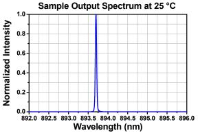
The apparent linewidth is limited by the measurement resolution, which is 7.5 GHz (0.25 cm<sup>-1</sup>)
