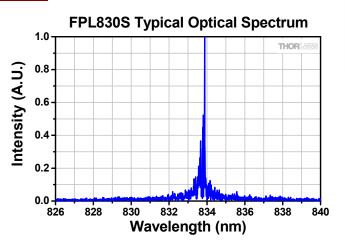
While the laser diode was held at 25 °C, it was driven at the current required to reach an output power of 350 mW.
