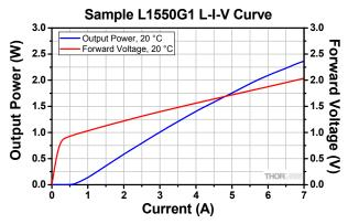
The data presented here is for one particular laser diode. Slight variations in performance data will occur from device to device. The sample spectrum and L-I-V spectrum of the L1550G1 laser diode was taken at 20°C. The far field was measured at a distance of 7" from the diode.
