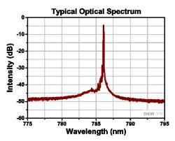
While the laser diode was held at 25 °C, it was driven at the current required to reach an output power of 250 mW.
