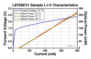
The typical output power vs. current is shown for three temperatures within the wavelength stabilized temperature range  $(\Delta T_{Stabilized})^*$  of a L976SEV1 laser diode.
