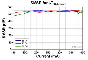
The typical side mode suppression ratio (SMSR) is shown for three temperatures within the wavelength stabilized temperature range  $(\Delta T_{Stabilized})^*$ .
