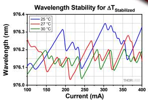
When used within the wavelength stabilized temperature range ( $\Delta T_{Stabilized}$ )\*, the L976SEV1 shows excellent wavelength stability over a range of drive currents.
