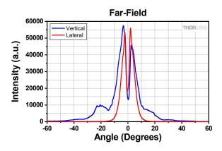
The diverging beam from the laser chip freely propagates through the external volume holographic grating (VHG), while the light in the center of the beam is reflected back into the chip. This results in a stabilized wavelength emitting from the laser and also creates a dark spot in the far field, as shown in the graphs above. These were measured with a current of 400 mA.
