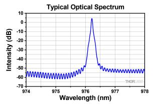
The typical optical spectrum is shown above. The data was obtained with a 350 mA drive current and the device held at 27° C.
