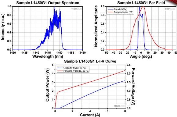
The data presented here is for one particular laser diode. Slight variations in performance data will occur from device to device. The sample spectrum and L-I-V spectrum of the L1450G1 laser diode was taken at 20°C. The far field was measured at a distance of 7" from the diode.
