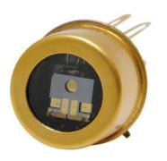
near-infrared light in the 0.85-1.7  $\mu$ m range. These detectors are hermetically sealed to ensure longevity. Within the detector package, a thermoelectric cooler is integrated with options of 1, 2, and 3 stages, as well as integration with a MEMS chopper, significantly reducing background noise while maintaining a compact format. Additionally, a driving PCB with an amplifier is available for convenient use.
