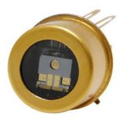
The CPOD serials lead selenide detectors (PbSs) provide enhanced sensitivity for detecting mid-infrared light in the 2-5  $\mu m$  range. These detectors are hermetically sealed to ensure low leakage. Within the detector package, a thermoelectric cooler and a MEMS chopper are integrated, significantly reducing background noise while maintaining a compact format. Additionally, a driving PCB with an amplifier is available for convenient use.
