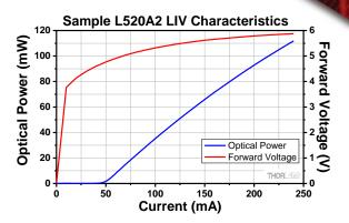
The data presented here is for one particular laser diode. Slight variations in performance data will occur from device to device. The sample spectrum of the L520A2 laser diode was measured at 15 °C, 25 °C, and 35 °C. The L-I-V characteristics data was taken at 25 °C. Please visit our website for raw spectral data and L-I-V characteristics.
