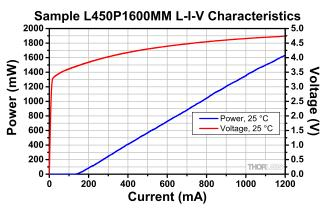
The data presented here is for one particular laser diode. Slight variations in performance data will occur from device to device. The sample spectrum of the L450P1600MM laser diode was measured at 10 °C, 25 °C, and 40 °C using a Thorlabs OSA201 Spectrum Analyzer with resolution of 7.5 GHz. The L-I-V characteristics data was taken at 25 °C. Please visit our website for raw spectral data and L-I-V characteristics.
