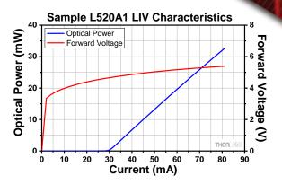
The data presented here is for one particular laser diode. Slight variations in performance data will occur from device to device. The sample spectrum of the L520A1 laser diode was measured at 15 °C, 25 °C, and 35 °C. The L-I-V characteristics data was taken at 25 °C. Please visit our website for raw spectral data and L-I-V characteristics.
