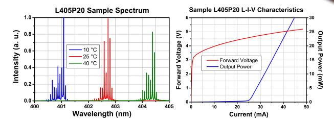
The data presented here is for one particular laser diode. Slight variations in performance data will occur from device to device. The sample spectrum of the L405P20 laser diode was taken at 10 °C, 25 °C, and 40 °C using a Thorlabs OSA201 Spectrum Analyzer with resolution of 7.5 GHz. The L-I-V characteristics data was taken at 25 °C. Please visit our website for raw data and L-I-V characteristics at 10 °C, 25 °C, and 40 °C.
