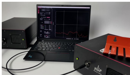
Sample 2. Reflection measurements of a painted metal plate.
