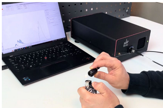
Measuring byproducts of combustion processes with NLIR's MIDWAVE Spectrometer in real time.
