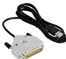
Compact digital I/O interface for USB remote control, supports opto-isolation of amplifier signal path from PC USB port, 16 digital outputs, 3 opto-isolated digital inputs, bus-powered operation
