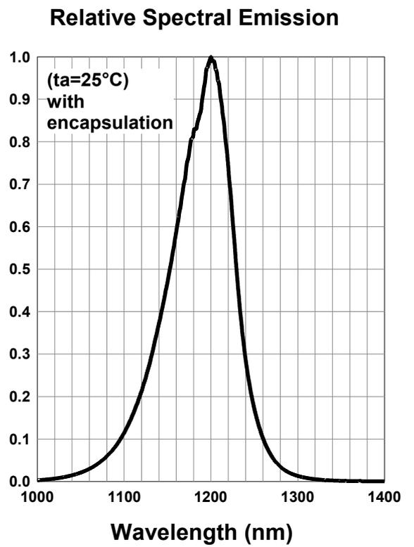
\*The absorption of lens resin changes spectral emission.
