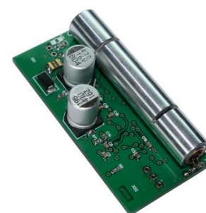
MDS-4 methane sensor module
