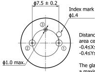
Distance from photosensitive area center to cap center  $-0.4 \le X \le +0.4$   $-0.4 \le Y \le +0.4$
