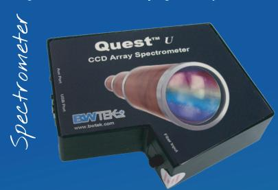
The Quest™ U (BRC112P-U) is a linear CCD array spectrometer optimized for UV performance using a low stray light optical bench. It features a 2048 element detector, built-in 16-bit digitizer, USB 2.0 interface with a >2.0 MHz readout speed, and external trigger. The Quest™ U is temperature compensated, which greatly reduces the thermal drift to ~15 counts/° C. This gives improved stability by decreasing baseline drift and sustaining the dynamic range.
