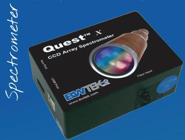
The Quest™ X (BRC112P-V) is a linear CCD array spectrometer optimized for UV and NIR performance using a low stray light optical bench. It features a 2048 element detector, built-in 16-bit digitizer, USB 2.0 interface with a >2.0 MHz readout speed, and external trigger. The Quest™ X is temperature compensated, which greatly reduces the thermal drift to ~15 counts/oC. This gives improved stability by decreasing baseline drift and sustaining the dynamic range.
