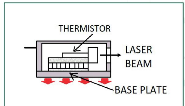
The above HHL-package diagram shows the built-in thermistor that monitors the laser chip temperature. The diagram also shows the base plate that dissipates the heat generated by the TEC and the laser chip.
