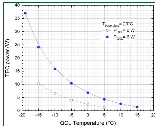
Power consumption of the built-in TEC<sup>1</sup> as a function of the QCL chip temperature for a base plate temperature of +20°C, with and without a thermal load in the QCL.
