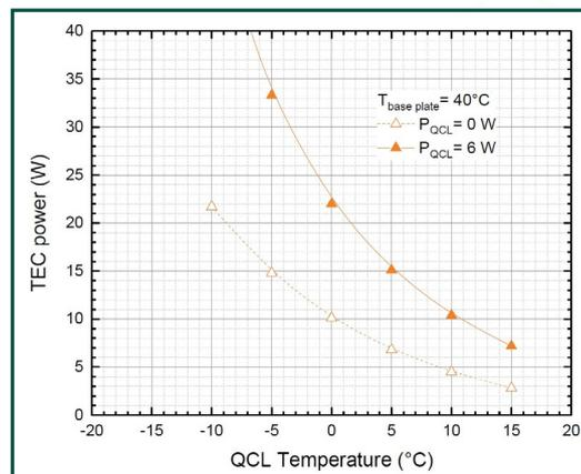
Power consumption of the built-in TEC<sup>1</sup> as a function of the QCL chip temperature for a base plate temperature of +40°C, with and without a thermal load in the QCL.
