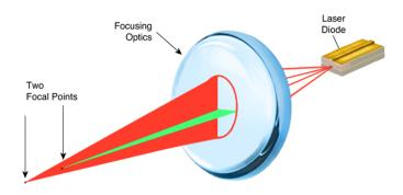
The diagram above illustrates the problems of astigmatism, and how it can limit your optical system performance in terms of focused beam shape and size. If precise beam placement or a small, focused image is required by your system, correcting astigmatism will improve your system performance.
