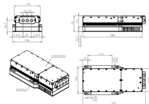
MPL2210 series laser head dimensions (in mm)
