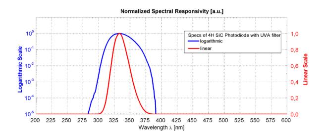
UVA-only SiC based UV photodiode A = 0.50 mm<sup>2</sup>
