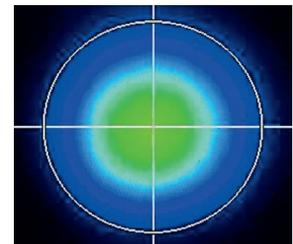
Typical beam intensity profile (20 cm from laser output) of MPL2310 series lasers
